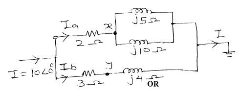
a) Find out voltage at node A and node B.
