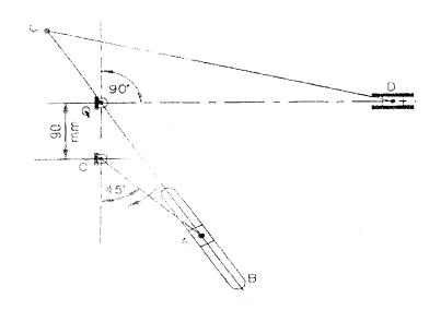
OQ = 90 mm, OA = 180 mm QC = 135 mm, CD = 450 mm. Speed of OA about O is 240 rpm uniform in the clockwise direction.
