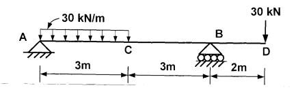
Q.3 Calculate the reactions R<sub>A</sub> & R<sub>B</sub>. Also, calculate shear force and bending moment at point D, using Influence Line Diagram. (10)
