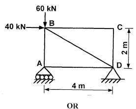
Q.2 Determine the horizontal deflection of joint B of the pin jointed truss as shown in figure, using Castigliano's first theorem. The area of each member is  $100 \text{ mm}^2$ . Take E = 210 GPa.
