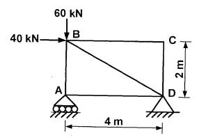
Q.3 Calculate the reactions R<sub>A</sub> & R<sub>B</sub>. Also, calculate shear force and bending moment at point C, using Influence Line Diagram. (10)
