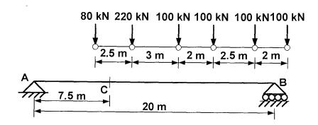
Q.4 Using Influence Line Diagram, calculate maximum bending moment at (10) point C for the beam as shown in figure.
