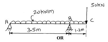
**Q.2** Draw shear force diagram and bending moment diagram for beam shown in [10] figure.
