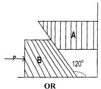
Calculate force F to maintain equilibrium. Take  $\mu$ =0.35 for all the surfaces. Q.2 Assume Pulley Frictionless.
