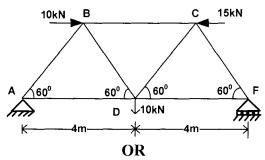
Q.3 Calculate forces in the member using method of joints and tabulate the answer. (10)
