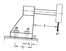
Q. 6 A welded connection as shown in fig. is subjected to an eccentric force of 8.5 (10) kN. Determine the size of welds if the permissible shear stress for the weld is  $115 N/mm^2$ . Assume static conditions.
