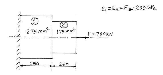
Calculate 1) Nodal displacement using element stiffness matrix 2) Elemental stresses 3) support reactions
