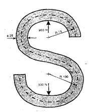
Q.7 Draw shear force and bending moment diagram for the beam shown
