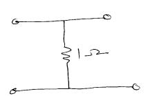
b) Show that the h parameters will not exist for a two port network when  $z_{22} = 0$ . [05]
