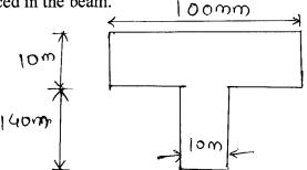
Q.4 Draw shear stress distribution on a T-section 160×15 mm deep (web) and 200×30 mm wide. The section is symmetric about vertical axis. The Shear force applied is 110KN.
