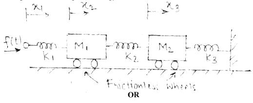
Q.1 a) Define transfer function. Derive transfer function of following:
