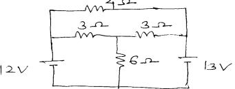
**b)** Using superposition find  $V_0$  of the shown network.
