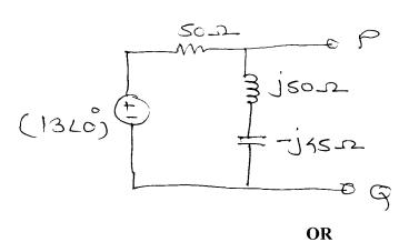
a) Write loop current equations for the shown network and determine current [05]
