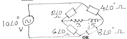
Q.1 a) Find Norton's equivalent circuit for network shown below at the left of (05) terminls 1-2 assume I=5< O Amp.
