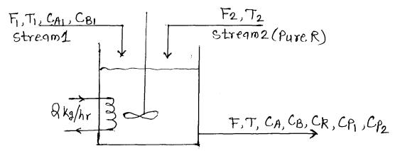
Both reactions are endothermic and both have second order Kinetics. Heat is supplied to the reaction mixture by steam which flows through a coil, immersed in the reactor, with heat transfer area  $A_t$ .
